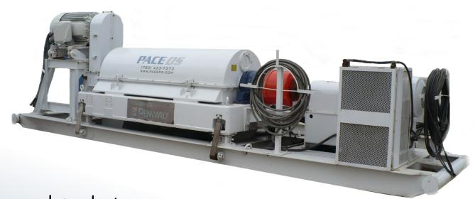
the Sharples PM-75,000 Super Decanter Centrifuge, stainless steel construction, single lead conveyor, adjustable liquid plate dams, 95:1 gearbox capable of 200 gallons per minute in municipal applications. This unit has a 250 hp main drive and 100 hp back drive.
